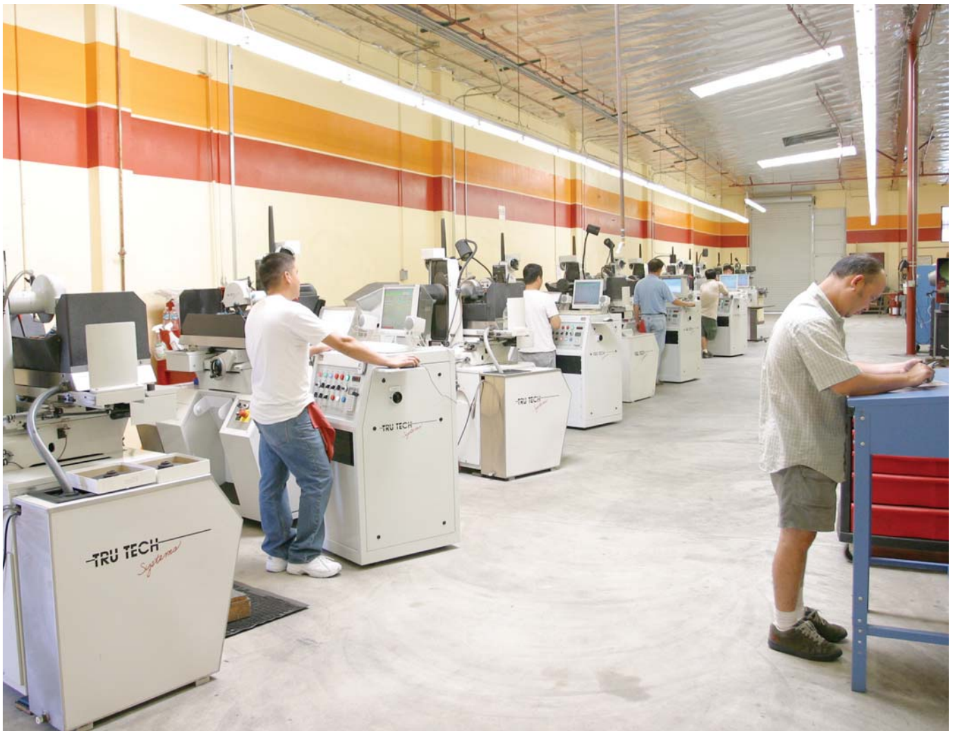
Lineup of Tru Tech centerless grinders at Helfer Tool Company in Santa Ana, California. The grinders work 20-22 hours a day producing precision custom tools for Helfer customers.
